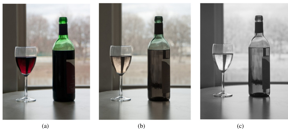
Figure 13. Images of a bottle and glass filled with red wine recorded for VIS light only (a), whole range VIS and NIR (b) and IR only (c).
