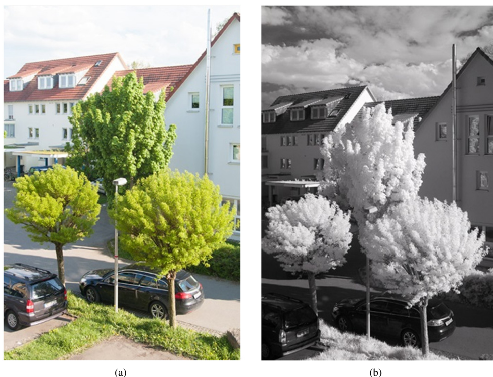
Figure 7. Another urban scene in VIS (a) and NIR (b) showing the same bright scattering effect of vegetation in the NIR. Note again the sky contrast and also the differences of reflection in the windows of the house on the right-hand side.
