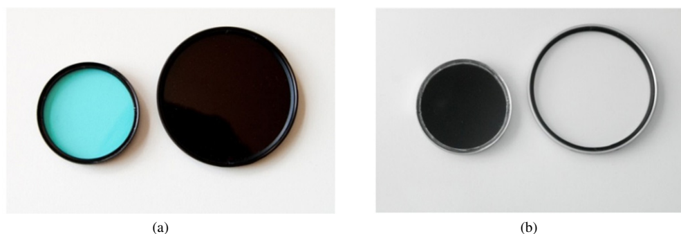
Figure 5. VIS (a) and NIR (b) photographs of two typical filters, the left one blocking NIR and the right one blocking VIS light.
